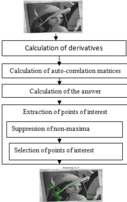
Fig. 1. Detection of points of interest by the Harris detector method.
