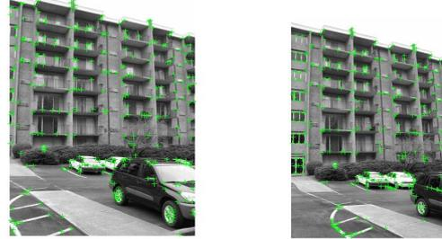
Fig. 4. Harris stereo images detector left and right.
