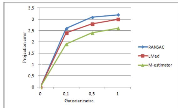
Fig. 6. Comparison of the proposed method projection error as a function of Gaussian noise.
