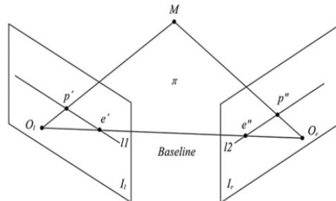
Fig. 2. Epipolar geometry of stereo images.
