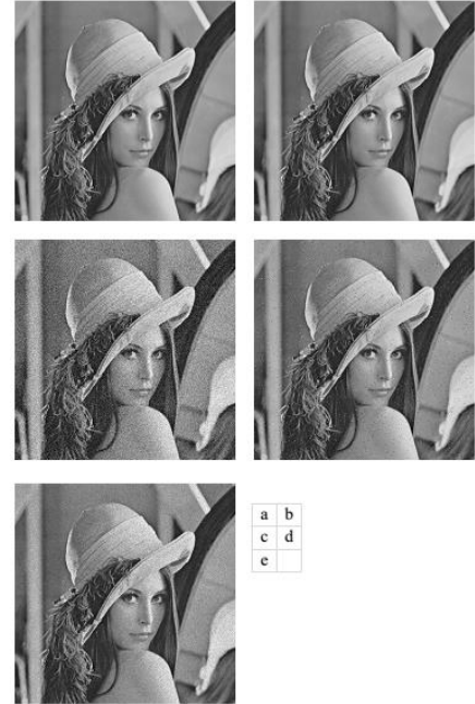
Fig. 6. (a) Host image Lena, (b) Watermarked image Lena, (c) Gaussian noise, (d) Salt &amp; Pepper noise, (e) Speckle noise.
