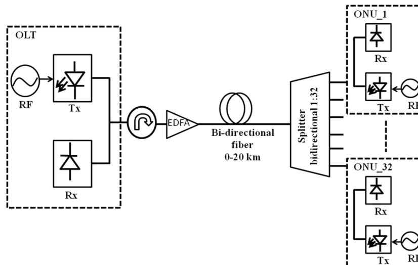
Fig. 4. Simulation set up in OptiSystem
