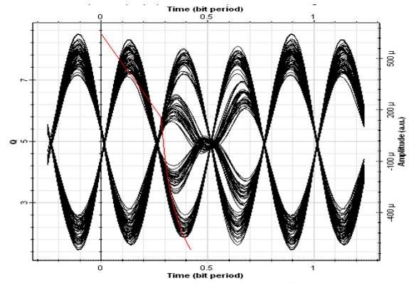
Fig. 7. Eye opening at 20 km fiber
