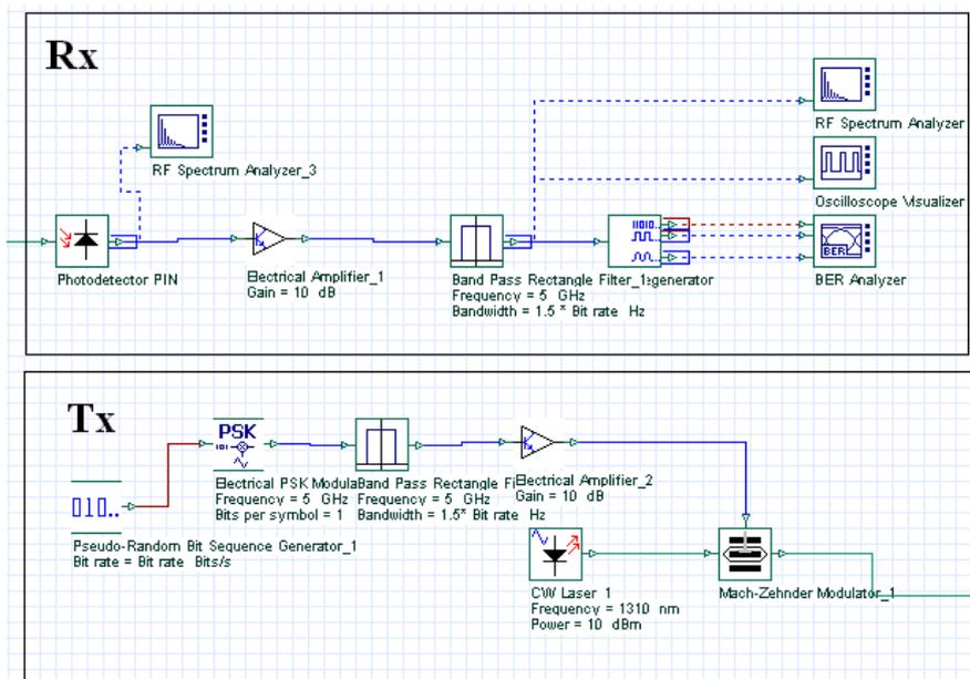
Fig. 5. Simulation set up in OptiSystem
