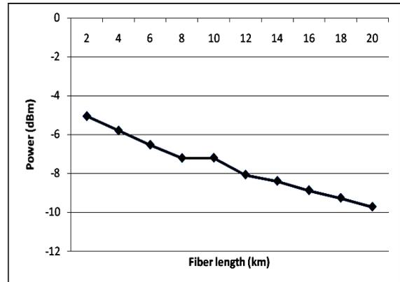
Fig. 11. Optical power at the Rx
