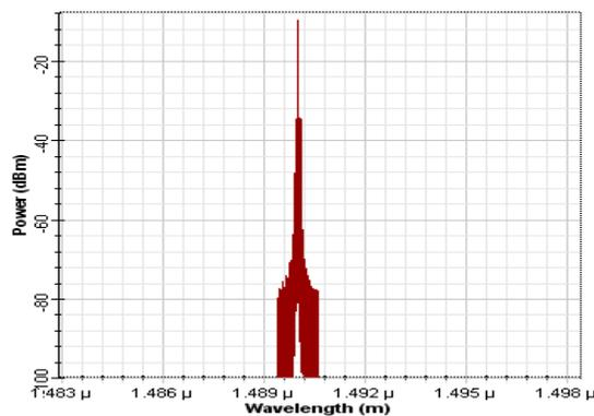
Fig. 10. Optical spectrum at Rx detection
