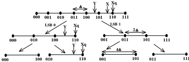
Fig. 2. The quantization bin [5]
