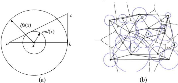
Fig.1. (a) Local feature size and minimum size, (b) Weighted Delaunay triangulation
