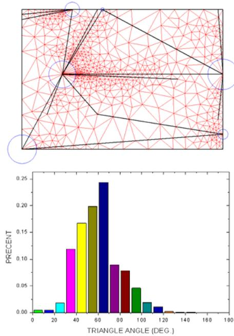
Fig. 7. Result meshes and plot of angle
