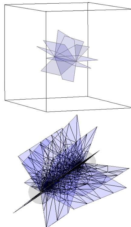
Fig. 9. No-manifold input PLC and resulting triangular mesh on the input facets
