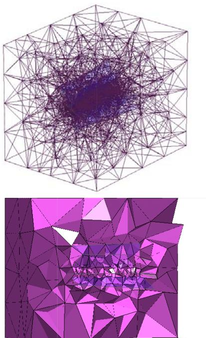
Fig. 10. Final tetrahedral mesh and a section view
