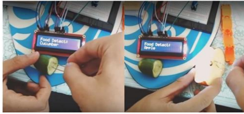
Fig. 5. Apple and cucumber detected by the device.
