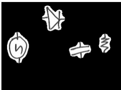
Fig. 6. Segmented components from Hand drawn circuit diagram.
