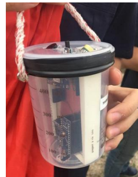
Fig. 3. The designed radiosonde configuration before a test.
