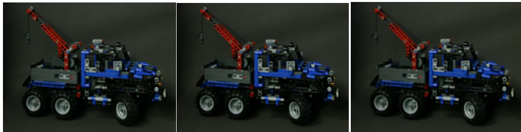
(a) Noncompressed (28.76dB) (b) Light field (i) (28.68dB) (c) Layer (ii) (28.64dB) Fig. 5. Reproduction results of center view without TDM at QP = 10 (Lego Truck).
