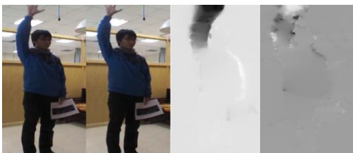
Fig. 6. From left to right: two consecutive frames and obtained optical flows in x and y directions respectively.
