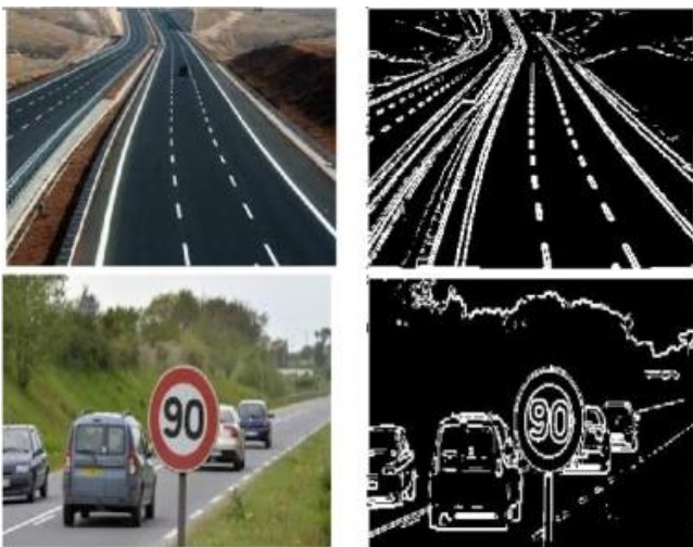
Fig. 2. Application of Laplacian algorithm to characterize different images
