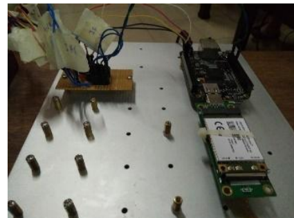
Fig. 8. The circuit on PCB connected with BeagleBone Black.
