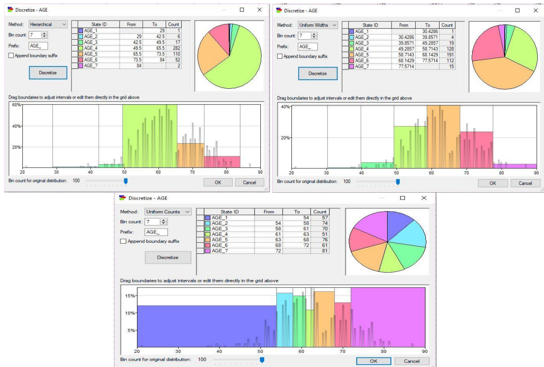
Fig. 5. Discretization statistics over AGE variable using 3 methods: hierarchical (top-left), uniform-width (top-right), and uniform-count (bottom).
