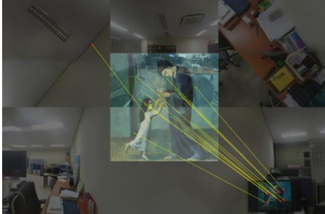
Fig. 16. Feature matching results when using ASIFT with two transforms (1, 2) for correct artwork.
