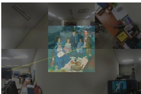
Fig. 19. Feature matching results when using ASIFT with five transforms (1-5) for a different artwork.
