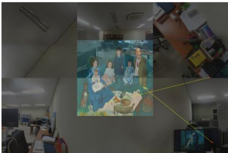
Fig. 17. Feature matching results when using ASIFT with two transforms (1, 2) for a different artwork.
