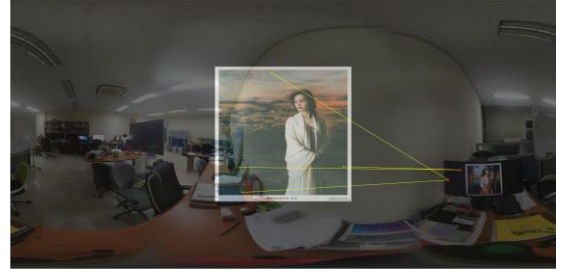
Fig. 7. Feature matches produced using UBCMATCH.
