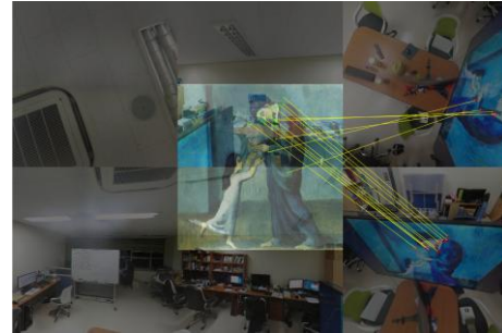
Fig. 20. Feature matching results when using standard ASIFT for correct artwork.
