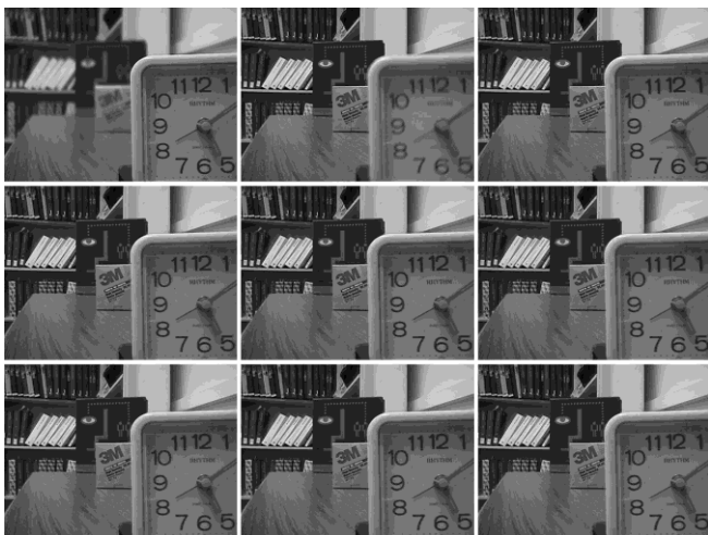
Fig. 4. The best results of “Table”: (top-row-left) first source image; (top-row-middle) second source image; (top-row-right) haar wavelet, DL = 2; (second-row-left) db20 wavelet, DL = 1; (second-row-middle) sym2 wavelet, DL = 1; (second-row-right) coif1 wavelet, DL = 2; (bottom-row-left) bior1.5, DL = 2; (bottom-row-middle) rbior1.5 wavelet, DL = 2; and (bottom-row-right) dmey wavelet, DL = 2.
