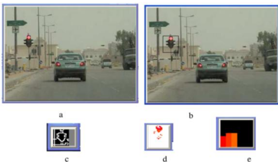
Fig. 12. The result of the recognition system on TL3 traffic light: (a) Original image, (b) The sliding window, (c) Reducing the image and applying canny algorithm, (d) Extracting the red color only, (e) Calculate the histogram.
