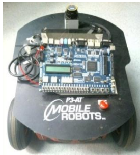
Fig. 5. Pioneer 3-AT with FPGA and LRF sensor.
