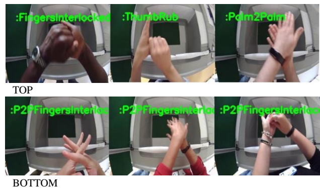
Fig. 8. Predictions for the sample frames with ResNet50 architecture. [Three at the Top are correct predictions (Set 2-50 epochs). Incorrect predictions at the bottom (Set 1-25 epochs)].
