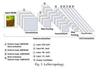
Finally, we flattened the image, getting a feature vector that is classified through connected layers as shown in Fig. 3. These connection layers are numbered from 5 to 8 and have tanh activation functions to raise the gap of the neuron weights. The last layer uses a softmax activation function [17] that estimates the class membership likelihood ("high," "middle," or "low").
