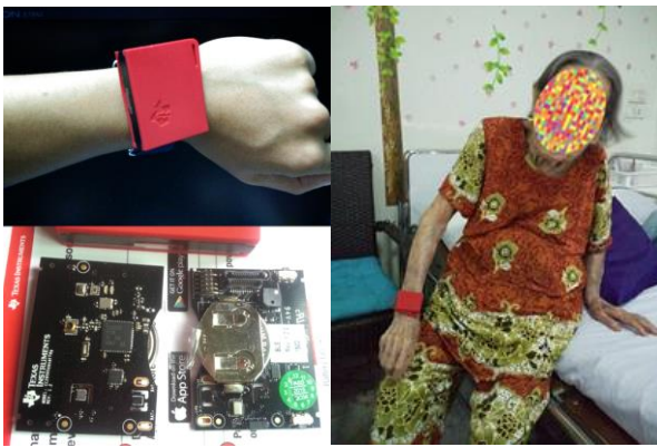
Fig. 2. TI sensor tag and the elderly wear the smart watch while doing a basic activity [4].
