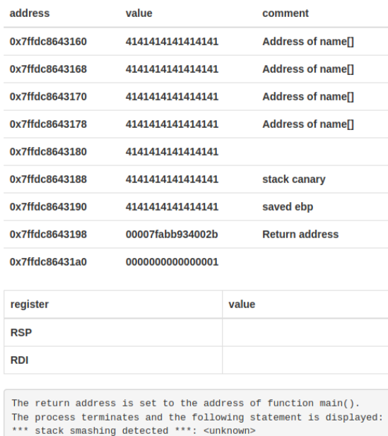
Fig. 8. A stack canary was overwritten by 0x4141414141414141 .
