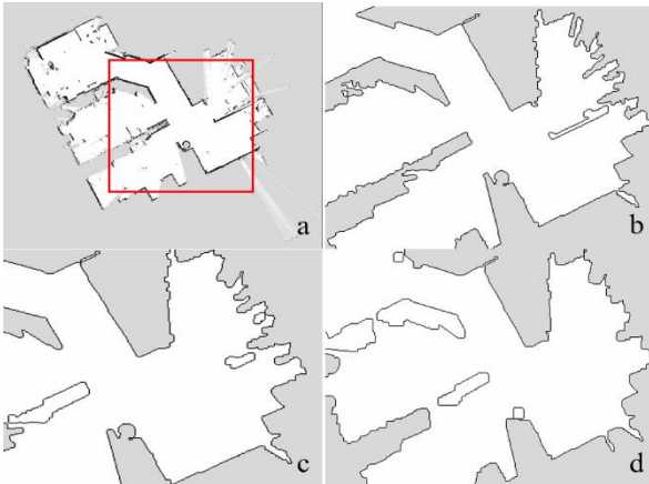
Fig. 9 Map improved by opening and closing operation. (a) Original image (b) Opening 3 \times 3 Closing 3 \times 3 (c) Opening 3 \times 3 Closing 5 \times 5 (d) Opening 3 \times 3 Closing 9 \times 9 .
