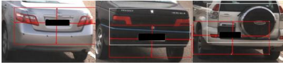
Fig. 4. Examples of 3 vehicle classes, Red Regions defined ROI relative to just license plate and white regions extracted optimal ROI by considering vehicle class.
