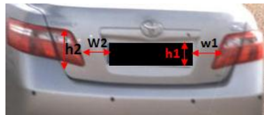
Fig. 3. Class of vehicle defined relative to location of license plate and taillights.
