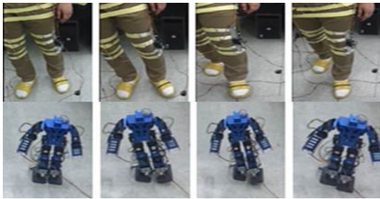
Fig. 6. the operator and the robot gait imitation control
