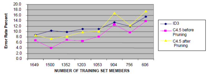
Chart 7. The error rate in Car data set, number of test set members is 149 and is fixed.
