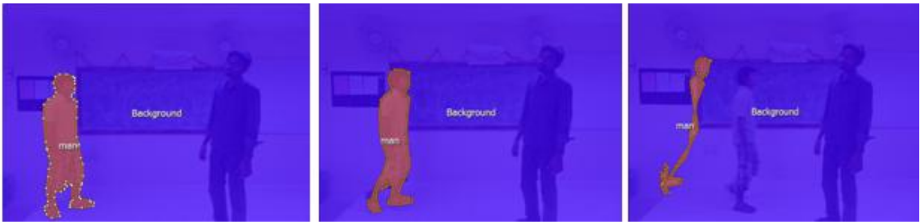
Fig. 6. Figure showing inability of contour tracking system on object deformation
