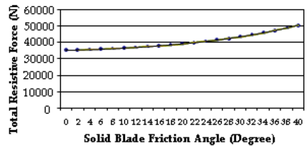
Fig. 5. Force vs. Solid blade friction angle.
