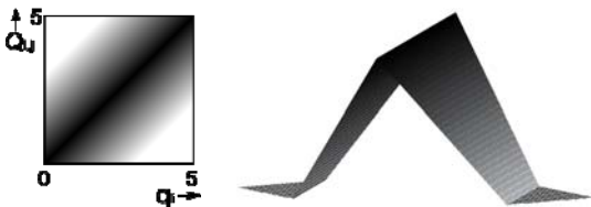
Fig 8. Linear kernel function where h = 3 . Topological view (left) and profile view (right).
